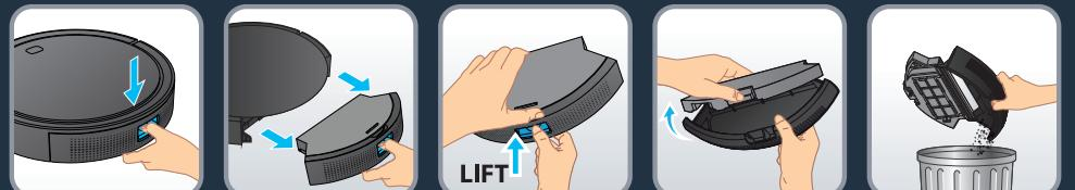
**EN** The robot must be emptied and cleaned after each use. Push the button on the backside of the robot and pull out the dust container. To empty it, flip off the cover.
