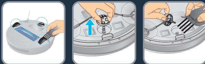
**EN** To clean the wheels, clean the front, left and right wheels regularly with a cleaning brush. The wheel shaft may be entangled by hair, cloth strips, etc. so please clean it in time.
