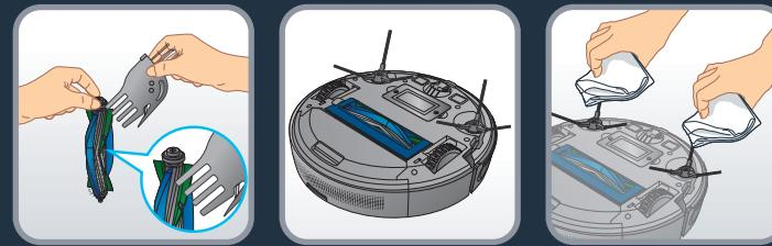
**EN** To clean the brush, use the cleaning accessory or scissors to cut away any hairs. Clean the robot's side brushes with a clean, dry cloth at least once a month.
