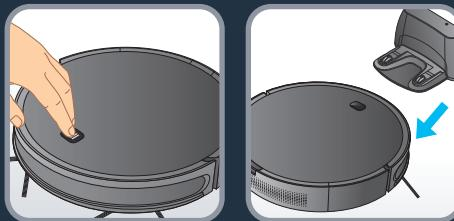
**EN** To clean all the accessible areas of your home, use the « Methodic » mode: press once the Power button. To clean a localized area of your home, use the « Spot » mode: press twice the Power button. Please note that the « Spot » mode is not available when the robot is on the docking station. To clean along the walls and in the corners, use the « Wall follow » mode: press three times the Power button.
