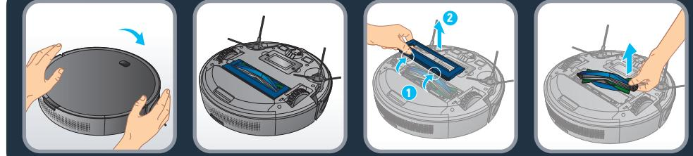
**EN** Clean the brush of the robot once a week. To do that turn the robot upside down. To remove the brush, open the brush guard by pushing the 2 snap latches and pull it up. Then pull out the brush from the robot.
