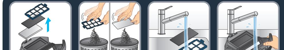
**EN** Clean the filter cover and the filter by tapping the back, holding it above a waste bin. Wash the foam filter, the filter cover and the dust catcher in clean water. Do not wet the fine dust filter (white filter). The filters must be cleaned at least once a week.
