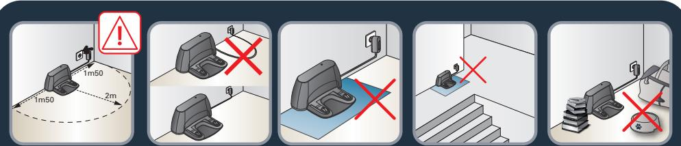
**EN** To place the docking station, make sure there is an empty area of 1.5m on each side and 2m in front of the docking station. Do not install the docking station near stairs. The cable must be tight. Always place the docking station on hard floor. Do not place the docking station on carpet.
